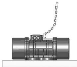
Figure3 Vibration motor anti-drop device
